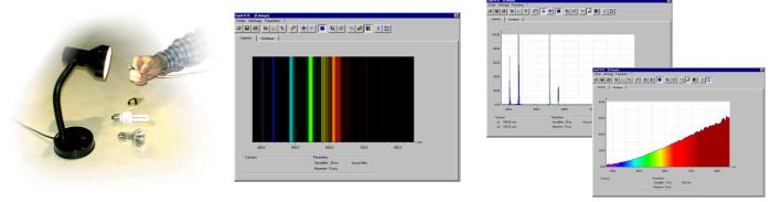
Spectrum of a « Energy saver » light source Spectrum of a mercury lamp and and of a incandescent light bulb
