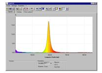
Transmission with an interference filter
