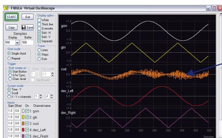
The Virtual Launch oscilloscope, with 1 to 8 channels has all the functionality of an oscilloscope hardware. The signals are labeled to visualize through probes.
