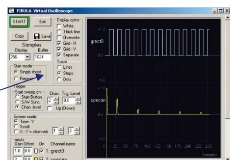
Spectral analysis, decomposition in Fourier series of a square wave.
