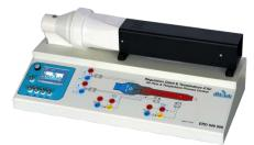
This process control enables a very progressive study of the control principles: Study of current loop - Experiment in current loop of air flow control or air temperature control.
