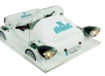
The **VMD** has been conceived for the sudy of a Local Industrial Network: CAN (Controller Area Networks). The model is based on the controls at the steering wheel in a car: light signalisation and windscreen wiper.
