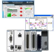
Control system based on National Instruments CompactRIO board with Input/Output modules adapted to Hydrelec 3E
