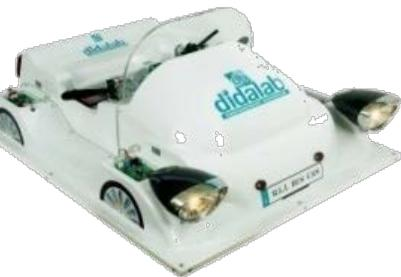
The **VMD** has been conceived for the study of a Local Industrial Network : CAN (Controller Area Networks). The model is based on the controls at the steering wheel in a car : light signalisation and windscreen wiper.
