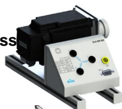
*Example of configuration : EL323 : 300 W motor bench, LV, 3-ph asynchronous squirrel motor coupled to a active load with mechanical values acquisition*
