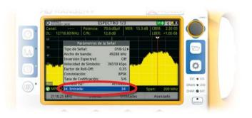
We can then enter a **specific stream identifier** that will be used by the analyser to recover the corresponding transport stream, service list and programmes data.
