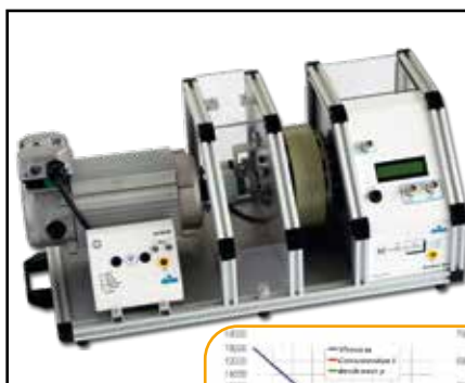
Torque speed relation DC motor (ELS 312 000)
