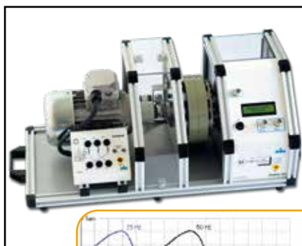
Torque speed relation 3-ph AC motor (ELS 313 000)
