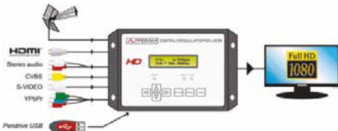
ETV 110 000 - Digital modulator, HD DTTV (EN206)
