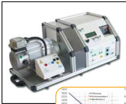
Torque speed relation DC motor (ELS 322 000)
