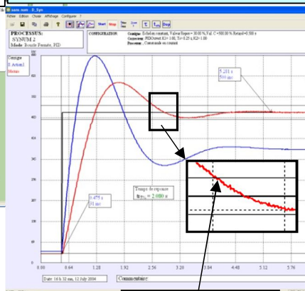
Automatic measurement of the response time at 5% on the feedback loop
