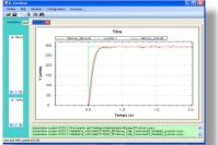
Validating the corrector by comparing of the results of the simulation and the experiment, and if necessary, adjusting the corrector, or searching another corrector with Scilab.
