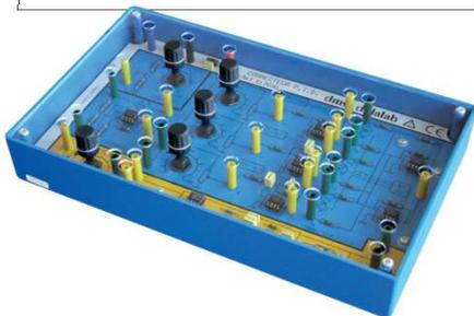
This module enables the study of the speed control of the DC rotating machine bench ref. 3788 & of the chopper.
