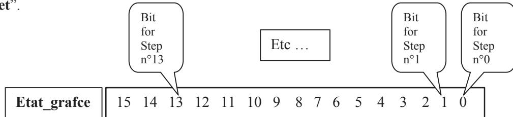
When a step is active, the linked bit is levelled at the logic state '1'. Of course, when a step is not active, it is levelled at '0'.
