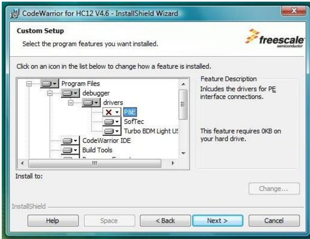
5. After the product has finished installing, plug in the SofTec In-Dart One using the supplied USB cable. Vista will prompt you to install the driver. Choose "Locate and Install driver software"
