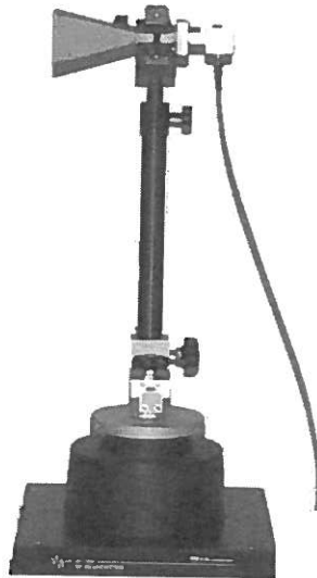
Figure 8-5 Setting of Even Polarization Horn Antenna
