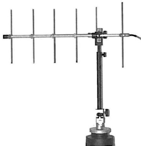
Figure 7-6 Setting of Vertical Polarization Transmitting Antenna
