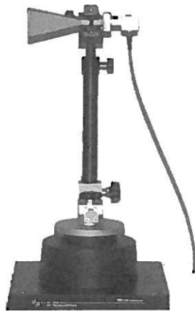
Figure 12-9 Horizontal Polarization Transmitting Antenna
