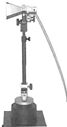
Figure 8-8 Rotation of Vertical Polarization Transmitting Antenna
