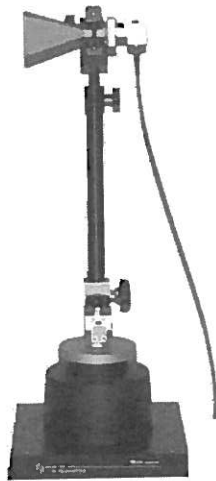
Figure 9-3 Setting of Even Polarization Horn Antenna
