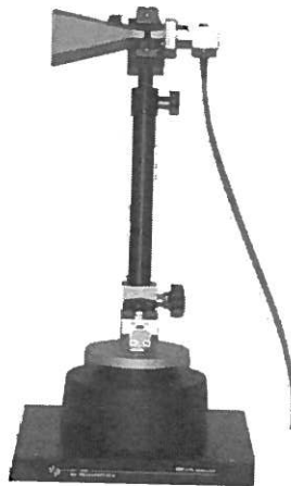
Figure 11-2 Setting of Even Polarization Transmitting Antenna
