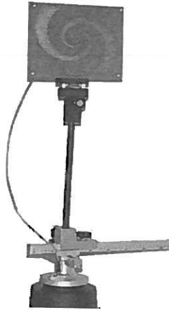
Figure 7-4 Setting of Even Polarization Receiving Antenna
