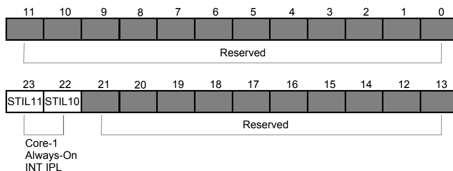
Figure 5-8. Core-1 Interrupt Priority Register P1
